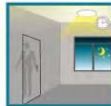
After hold time, the sensor dims the lamp at a low light level if no new motion trigger.
