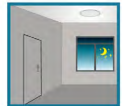
After stand-by period, the sensor switches off the lamp if no motion is detected in its detection zone.
